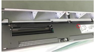
80XX-UH: Slide and open the panel, a black button on the inside like the figure shown below.
