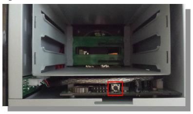
50XX-UH/UT: Slide and open the panel, a black button on the inside like the figure shown below.
