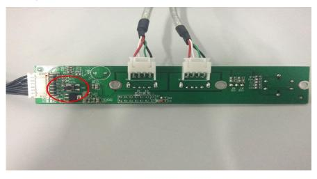
70XX-UH: Slide and open the panel, a black button on the inside like the figure shown below.
